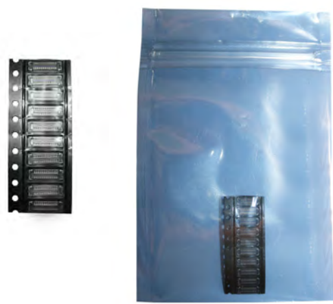
Place Connectors into Reel
